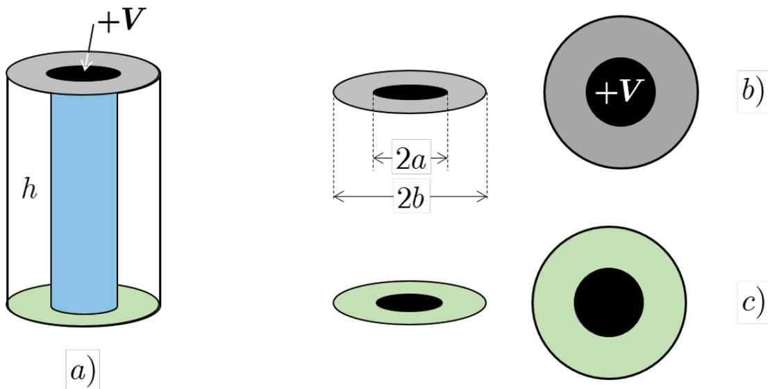
Figure 4: geometry of the battery a), coaxial cable b), and resistor c)
